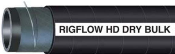
Series 8089 RIGFLOW Dry Material Suction Hose is designed to transfer dry abrasive materials. The tube is 3/16" thick for maximum abrasion resistance.
