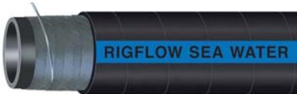
Series 8054 RIGFLOW Heavy Duty Sea Water Hose is designed to handle a wide range of applications in general industry, construction, agriculture and sea water applications. The tough, flexible EPDM rubber construction resists abrasion, weathering, UV and agricultural herbicides and other mild chemicals. The hose incorporates a steel wire helix for full suction capabilities, and multiple high tensile textile plies for discharge pressure.
